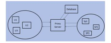
As mentioned in the diagram user gives request to proxy server. Proxy server checks and authenticates the user. After verification the service request is sent to the CSP and the service is provided to the user through the proxy server.
